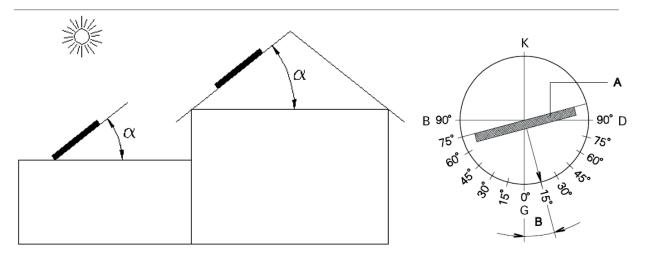
A- Collector deflection B- Azimut Angle
