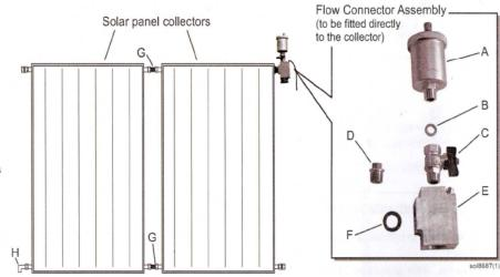
For Pitched Roof Only: The Automatic Air Vent must be installed internally at a level above that of the collectors (i.e. within the pitch of the roof) to allow access for manual venting from within the roof space.
